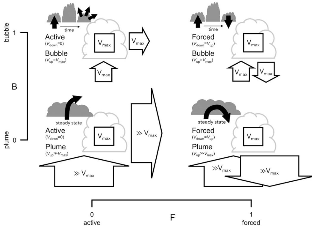
FIG. 1. The four extreme cases of a shallow cumulus cloud: (top left) an active bubble with  $F \equiv V_{\text{down}}/V_{\text{up}} = 0$  and  $B \equiv V_{\text{max}}/V_{\text{up}} = 1$ , (top right) a forced bubble with  $F = 1$  and  $B = 1$ , (bottom left) an active plume with  $F = 0$  and  $B = 0$ , and (bottom right) a forced plume with  $F = 1$  and  $B = 0$ .
