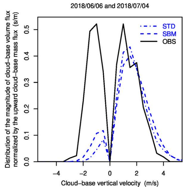
FIG. 9. Normalized distributions of the magnitude of cloud-base volume flux for STD (dashed-dotted blue), SBM (dashed blue), and OBS (solid black). Each distribution has been normalized by the integral over positive cloud-base vertical velocity (i.e., normalized by the gross ascending volume flux).
