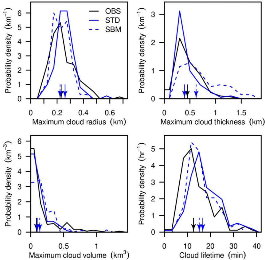
FIG. 2. The distributions of individual clouds among the datasets of OBS (black), STD (solid blue), and SBM (dashed blue) as functions of the cloud’s (top left) maximum effective radius, (top right) maximum thickness, (bottom left) maximum volume, and (bottom right) lifetime. The curves for STD and SBM are generated from 70 clouds (35 for 6 Jun 2008 and 35 for 4 Jul 2008) and the curves for OBS are generated from 158 clouds collected over 12 different days. Arrows indicate the median values.
