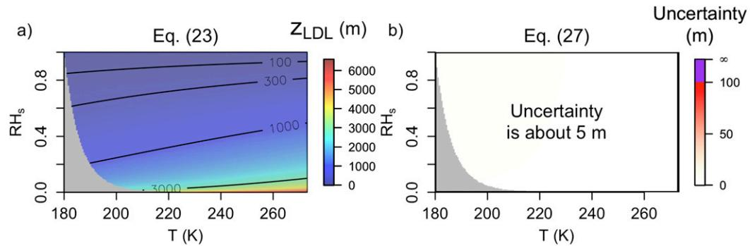
FIG. 4. (a) Contours of  $z_{LDL}$  from the exact Eq. (23) plotted for  $z = 0, p = 1$  bar, for all temperatures between 180 and 273 K, and all surface relative humidities from 0% to 100% with respect to solid water. The gray region marks the combinations of  $T$  and  $RH_s$  for which  $T_{LDL} < 180$  K, below which we do not have empirical measurements of  $p_v^{*s}$ . (b) The uncertainties from Eq. (27).
