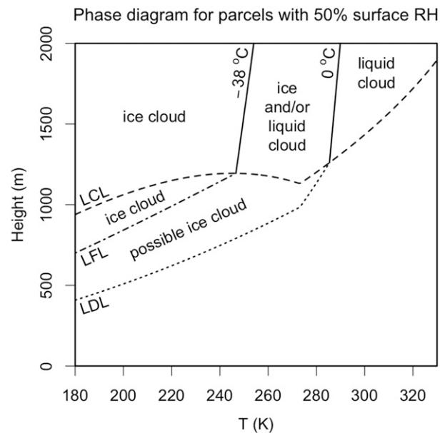
FIG. 2. For surface air with an RH of 50% with respect to liquid for  $T \geq 0^\circ\text{C}$  and with respect to solid (i.e., ice) for  $T < 0^\circ\text{C}$ , the LCL from Eq. (22) (dashed), LDL from Eq. (23) (dotted), and LFL from Eq. (25) (dash-dotted). The solid curves labeled  $0^\circ$  and  $-38^\circ\text{C}$  are the parcel isotherms calculated assuming liquid-cloud moist adiabatic ascent above the LCL.
