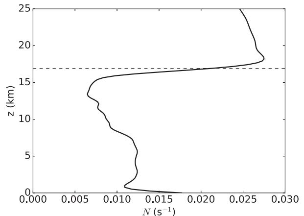
FIG. 2. Mean profile of the Brunt-Väisälä frequency  $N$  calculated from soundings taken every 3 h at the Darwin ARM site from 18 Jan to 3 Feb 2006. The dashed line denotes the cold-point tropopause at 16.9 km.
