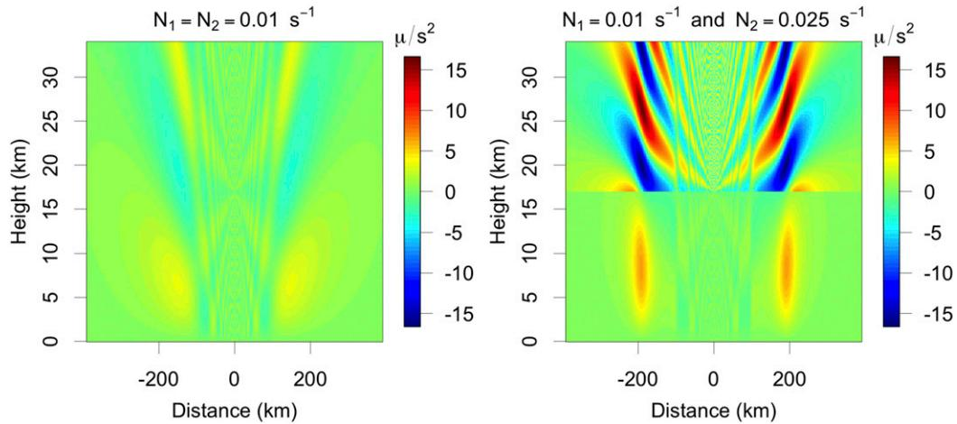
FIG. 3. (left) The no-lid solution  $b_m^{\text{no-lid}}$  at  $t = 1$  h in an atmosphere with  $N_1 = N_2 = 0.01 \text{ s}^{-1}$  that was subjected to the heating given by Eq. (8) with  $H = 17$  km,  $m = \pi/H$ , and  $B_0 = 1 \text{ m}^2 \text{ s}^{-2}$ . (right) As in (left), but for  $b_m^{\text{leaky}}$  with  $N_1 = 0.01 \text{ s}^{-1}$  and  $N_2 = 0.025 \text{ s}^{-1}$ .
