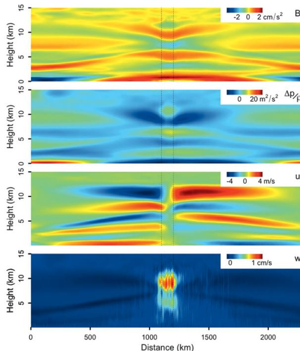
FIG. 1. For the bowling-alley simulation with a 100-km hot spot, the average (over 8 km of  $y$  and 1 month) of (top to bottom) buoyancy  $B = (\langle\rho\rangle/\rho - 1)g$ , pressure perturbation  $(p - \langle p\rangle)/\langle\rho\rangle$ , horizontal velocity  $u$ , and vertical velocity  $w$ , where angled brackets denote an additional average over  $x$ . Axes are  $x$  and  $z$ , and vertical dotted lines denote the boundaries of a 100-km-wide column.
