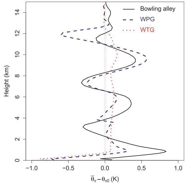
FIG. 4. Steady-state anomaly in virtual potential temperature for the bowling-alley column (black), WPG with  $1/\alpha^* = 10$  h (dashed blue), and WTG with  $\tau = 5$  min (dotted red). The anomaly is calculated with respect to the average over the entire bowling alley.
