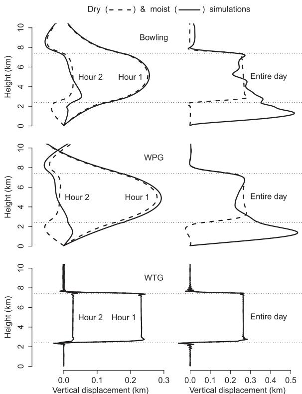
FIG. 8. Net vertical displacements (integrals over time of vertical velocity) for the (top) bowling alley, (middle) WPG, and (bottom) WTG. (left) The net displacements generated during the first and second hours to give a sense of the temporal evolution of the column. (right) The net displacement during the entire day. Dashed curves are from the dry simulations and solid curves are from the simulations with lower-tropospheric humidity.
