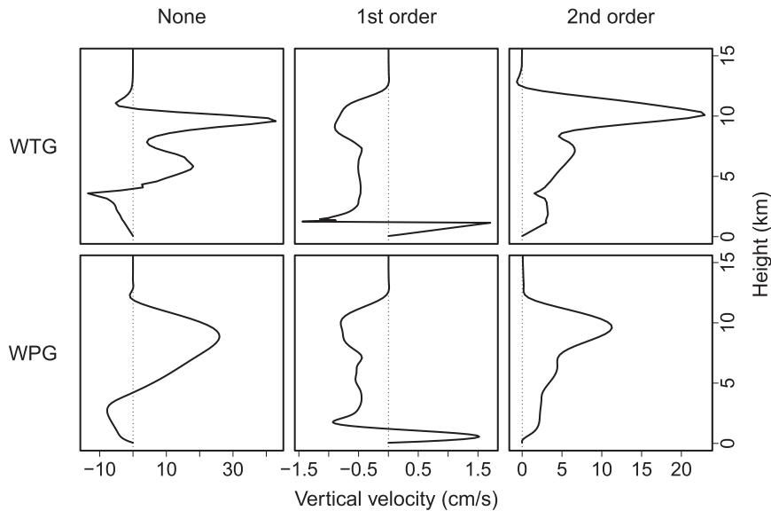
FIG. 5. Steady-state vertical-velocity profiles using (top) WTG and (bottom) WPG for three different treatments of horizontal advection due to convergence: (left to right) none, first order, and second order.
